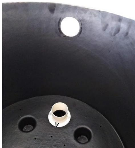
Align the socket in the tray marked 'V' with the vent hole cut in the side. Slide the Vent pipe marked 'V' into the socket. Slot fully in, until the pipe reaches the bottom, and the threaded part of the fitting slides out through the vent hole. From the outside, slide on the supplied seal, and hand tighten the supplied female fitting to the thread. Make sure the seal stays reasonably central whilst doing this.
